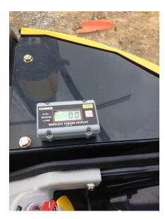
CHANCE Digital Torque Indicator mounted between the drive head and anchor tool (L). Wireless display mounted on the installation equipment to allow the operator to continually monitor torque (R).
